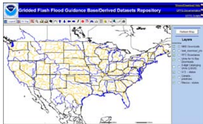
The GFFG Base-Derived Datasets Repository. Yellow features indicate the relatively large hydrologic units by which the datasets will be organized and downloadable, and blue features represent the RFC boundaries.
