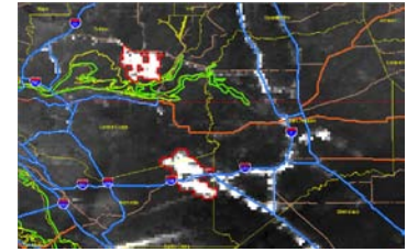
Red polygons delineate Q2 hot spot areas that coincide with large wind farms. Note that highways can also be a source of radar interference.
