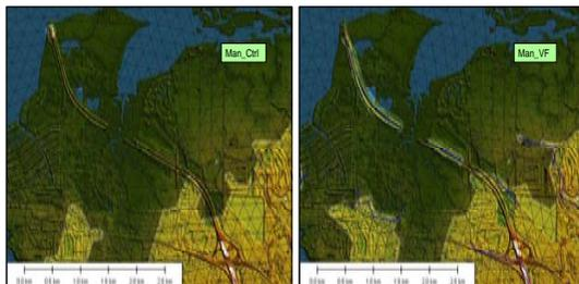
Inundation areas (shaded) for Man\_Ctrl (from a control mesh) and Man\_VF (from a mesh that defines particular vertical features, shown in blue) in the area of Interstate-75 on the southern bank of the Manatee River
