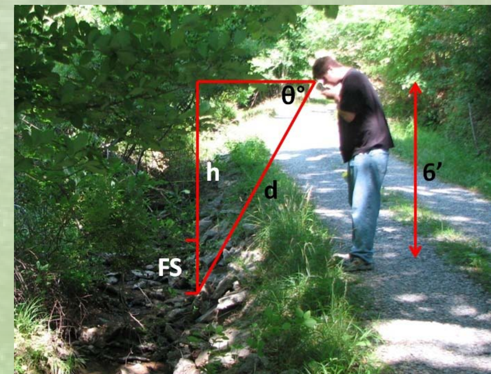
Figure 3. Diagram showing how flood stage (FS) is calculated.
